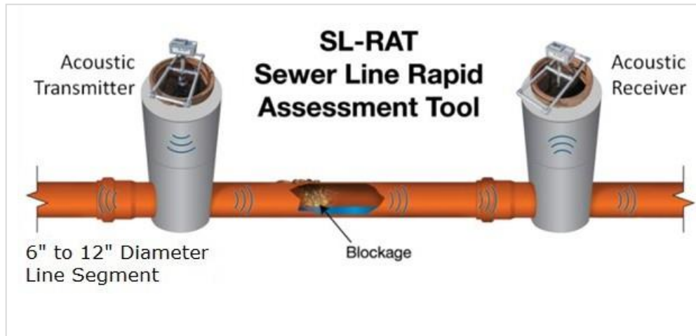
Figure 7. SL-RAT Concept and Operational Procedure
