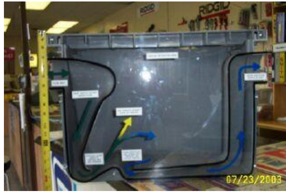
Cut away view of plastic Grease Interceptor design with special inlet and outlet baffle. This is a 20 gpm / 40 pound GT and is approximately 15 inches deep, and 24 inches long.
